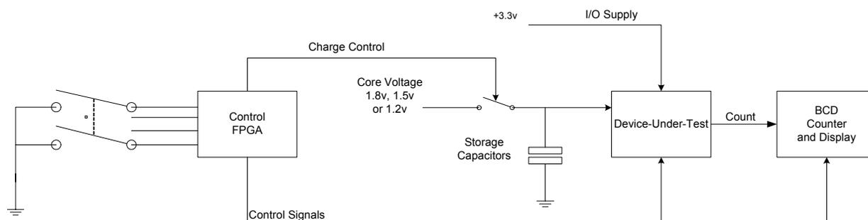
To enable users to test power consumption at different frequencies, the Power Demo Board's DIP switch SW2 applies a 4-bit code to the control FPGA that divides the master oscillator's 25 MHz reference frequency by 16, 32, 512, or 8,192. These division ratios apply nominal clock frequencies to the DUTs of 1.5625 MHz, 781.25 kHz, 48.828 kHz, and 3.052 kHz. Sockets allow users to substitute oscillator modules of their choice.
