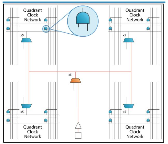
Figure 27-8: FPGA Clock Architecture
