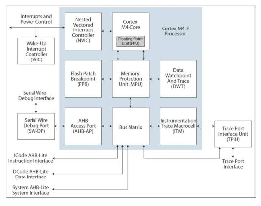
Figure 3-4: NVIC in S3 system architecture
