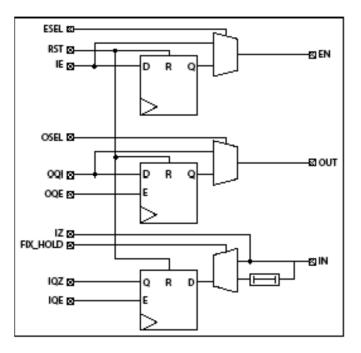
Figure 27-12: On-Chip Programmable Logic Configurable Input/Output
