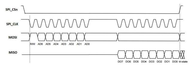
Figure 25-4: Basic SPI Read Operation (mode 11)
