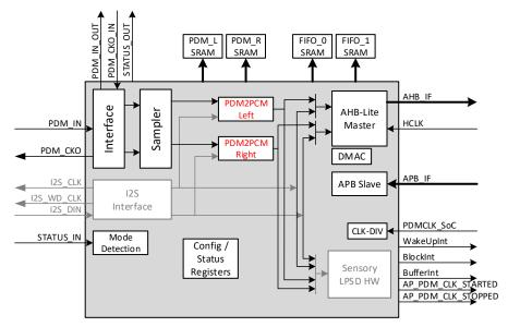
Figure 20-5: Voice / audio processing sub-system PDM VoiceQ Mode
