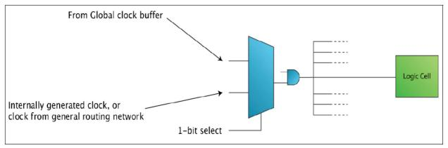
Figure 27-11: Quadrant Clock Structure
