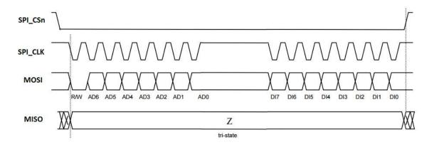
Figure 25-3: Basic SPI Write Operation (mode 11)
