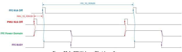
Figure 32-4: FFE Wake up/Shutdown Sequence
