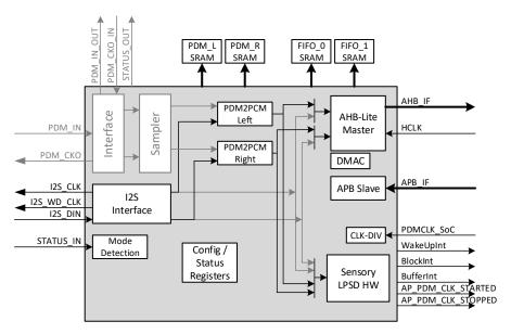
Figure 20-7: Voice / audio processing sub-system I<sup>2</sup>S Sub-Sample Mode
