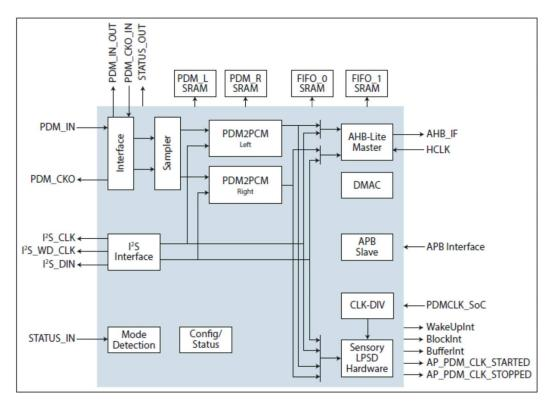
Figure 6-1: VP DMAC in the Voice / audio processor
