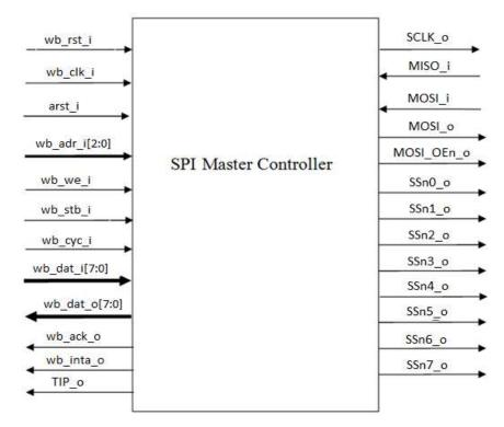
Figure 25-1: SPI\_0\_Master block connections
