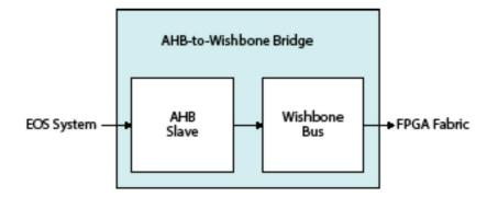
Figure 27-14: AHB-to-Wishbone Bridge
