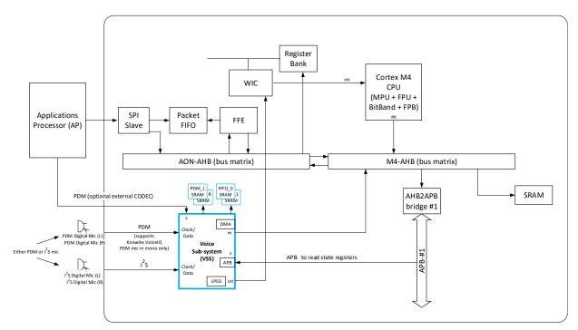
Figure 20-1: Voice / audio processing sub-system used in a design with Applications Processor
