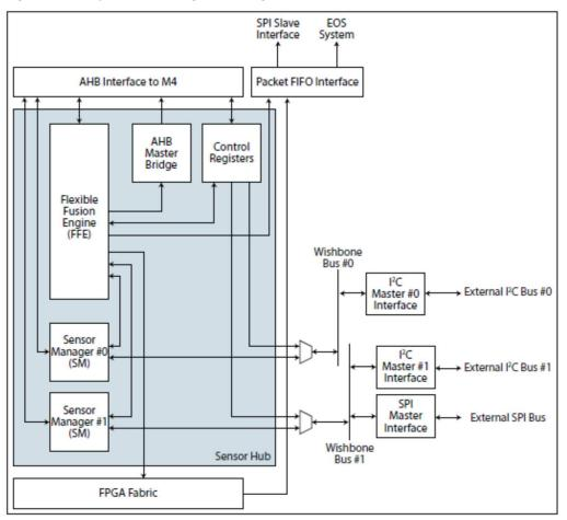
Figure 24-3: SensorHub subsystem with Wishbone buses
