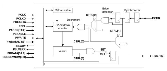
Figure 3-5: M4 Timer Block Diagram
