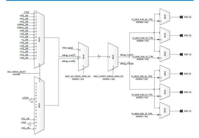
Figure 37-1: Clock Debug Multiplexers
