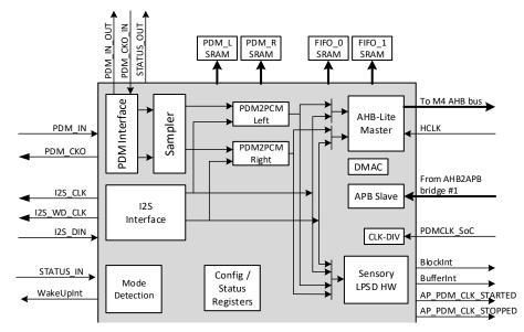
Figure 20-2: Voice / Audio Processing sub-system internal block diagram
