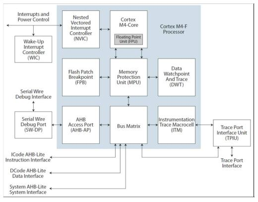
Figure 3-2: Cortex-M4-F Block Diagram
