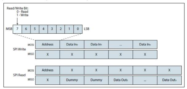
Figure 14-2 shows an example of the SPI Interface protocol. In each case, the MSB bit is shifted out first.
