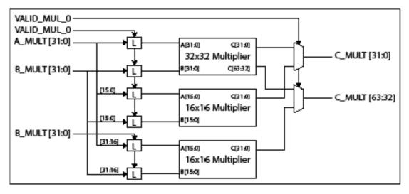
Figure 27-13: On-Chip Programmable Logic Multiplier
