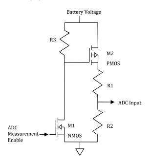
Figure 18-2: Example Voltage Divider Circuit
