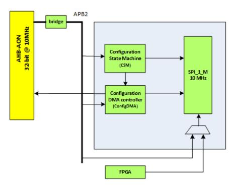
Figure 33-1: Configuration Manager high-level architecture
