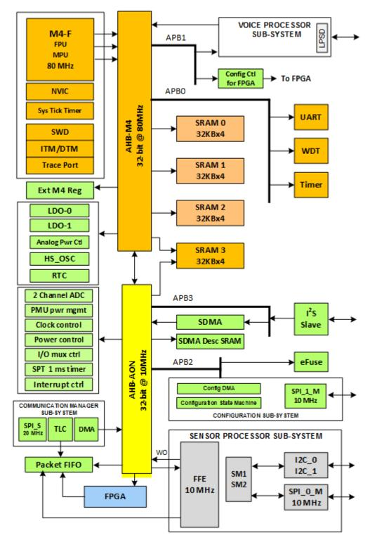
Figure 2-1: S3 high-level block diagram, with five main sub-system groups color coded
