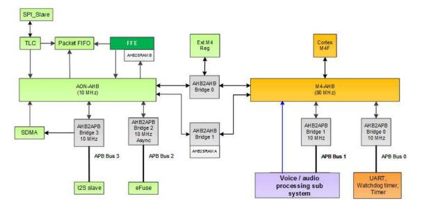
Figure 2-2: Bus architecture in S3
