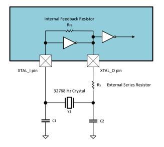
Figure 10-1: 32768 Hz crystal oscillator circuit
