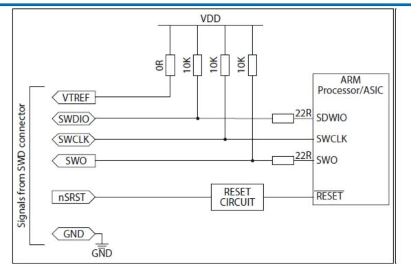
Figure 28-1: Recommended External Debugger Connection for ARM DS Debugger
