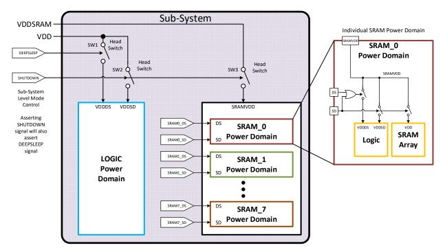
Figure 32-1: Logic and SRAM Power Domains within a Sub-System
