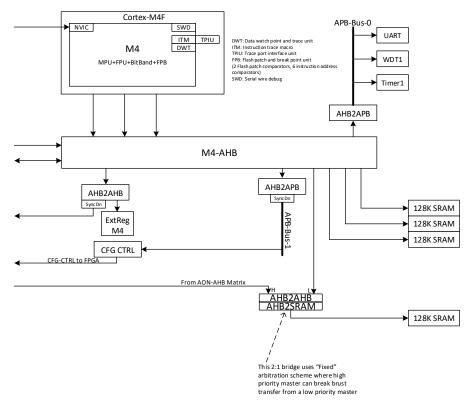
Figure 3-1: Cortex-M4-F sub-system Block Diagram
