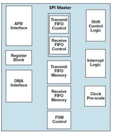
Figure 34-1: SPI Master Block Diagram
