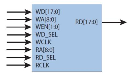
Figure 27-2: 8Kbit Dual Port RAM block in 512x18 configuration
