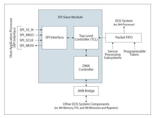
Figure 14-1: SPI\_Slave within the Communication Manager
