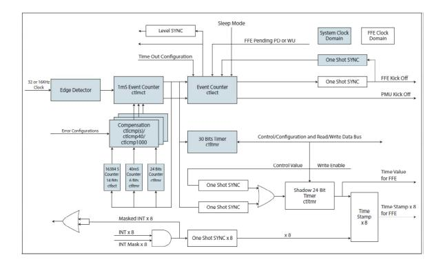
Figure 16-1: SPT Block Diagram
