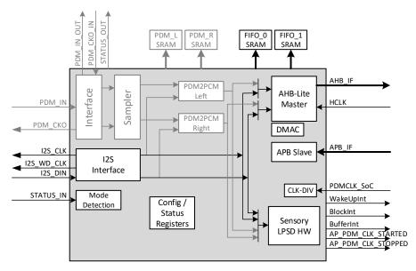
Figure 20-6: Voice / audio processing sub-system I<sup>2</sup>S Direct Mode
