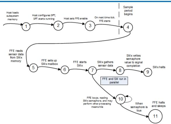
Figure 22-1: General flow of states in the Sensor Hub
