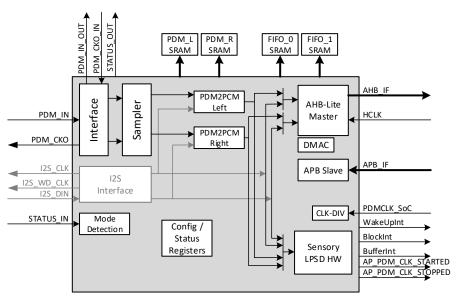
Figure 20-4: Voice / audio processing sub-system PDM External CODEC Mode
