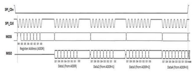
Figure 25-5: SPI Multiple Read Operation (mode 11)
