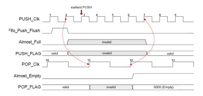
Figure 27-6: FIFO Flush from PUSH side
