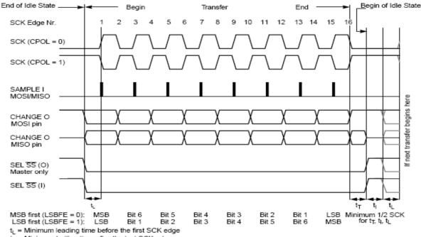
t<sub>T</sub> = Minimum trailing time after the last SCK edge
