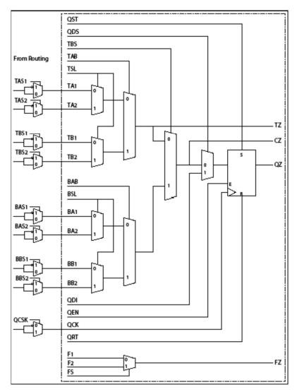
Figure 27-1: Logic Cell Block Diagram
