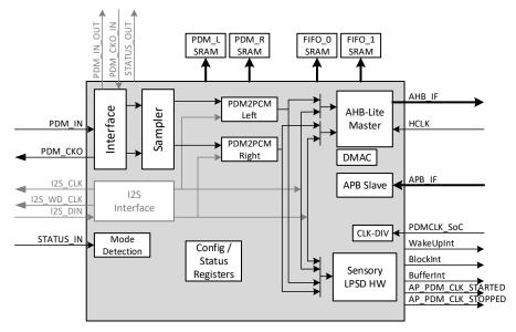
Figure 20-3: Voice / audio processing sub-system PDM Internal CODEC Mode
