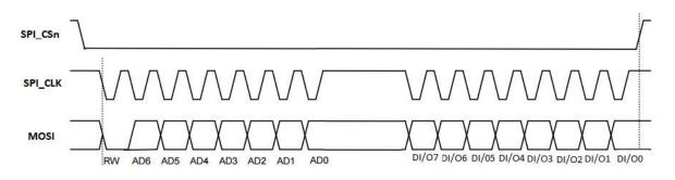
Figure 25-6: 3-wire basic SPI read / write sequence (mode 11)
