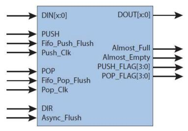
Figure 27-5: eFPGA FIFO Module
