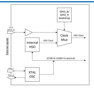
Figure 30-1: Selecting either internal or external High Speed Oscillator (HSO)
