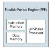
Figure 23-1: FFE block diagram
