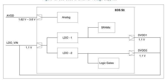
Figure 42: Use Case 3: External Voltage Supplied
