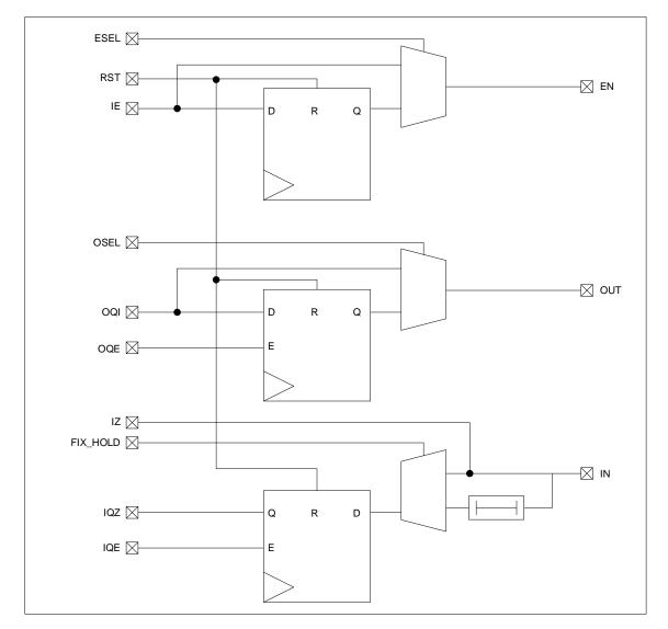
Figure 37: On-Chip Programmable Logic Configurable Input/Output
