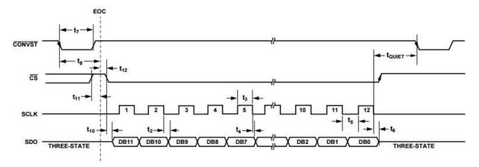
Figure 24: AD7091 SPI Transfer Sequence
