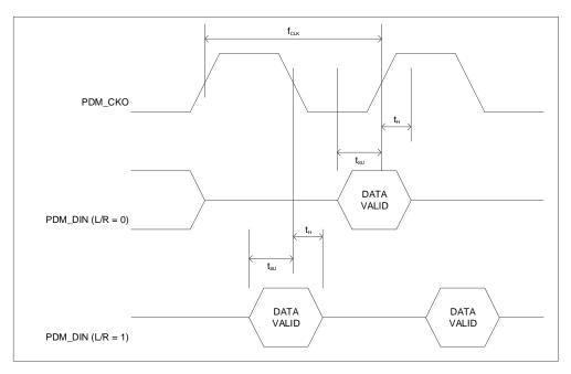
Figure 33: PDM Microphone Timing
