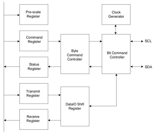
Figure 10: I2C Block Diagram
