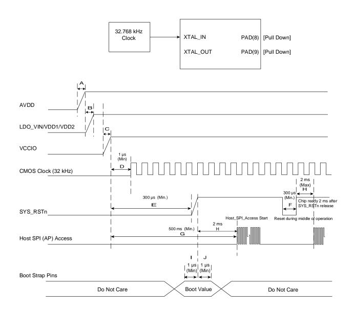
The following figure shows the power-on sequencing timing parameters.
