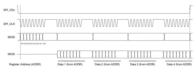
Figure 21: SPI Multiple Read Operation (Mode 11)
