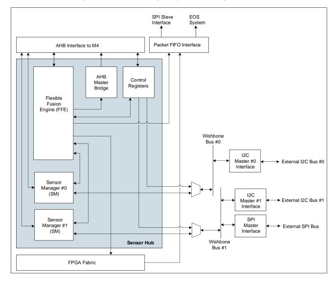
Figure 5: Sensor Processing Subsystem Block Diagram
