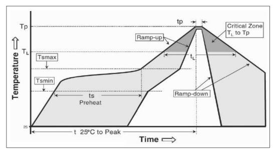
Figure 63: Pb-Free Component Preconditioning Reflow Profile
