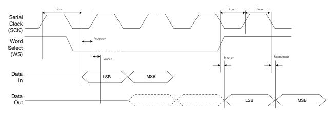
Figure 32: I<sup>2</sup>S Timing Waveform
