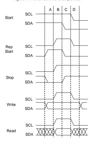
Figure 11: I<sup>2</sup>C Bit Command Sequences
