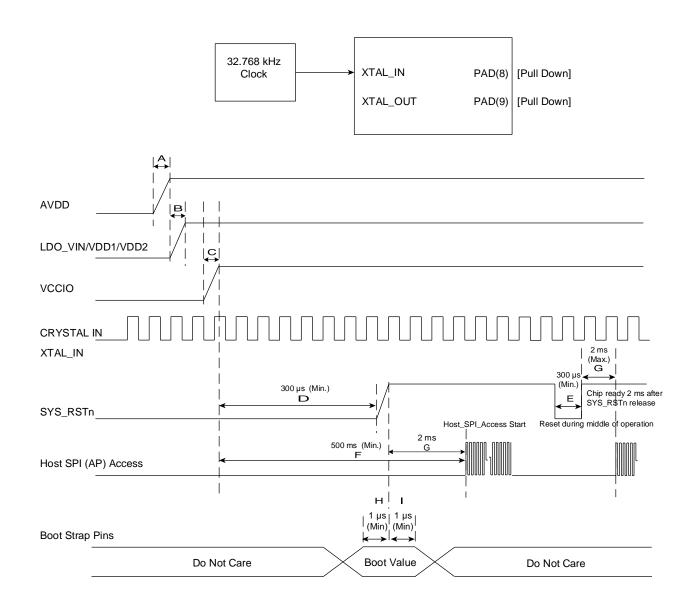
The following figure shows the power-on sequence timing parameters.
