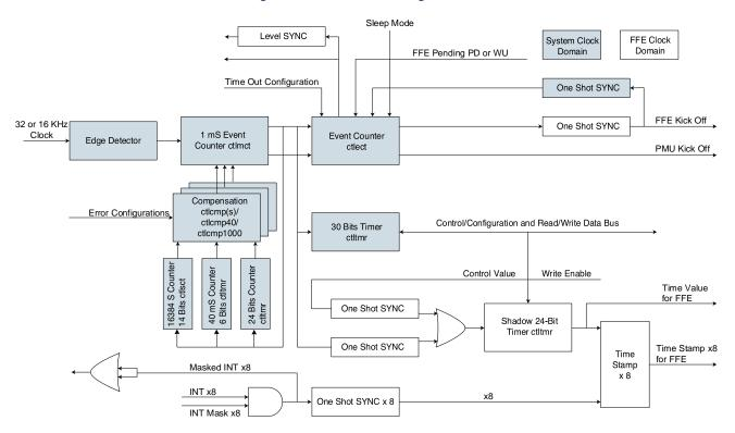
Figure 55: Timer Block Diagram
