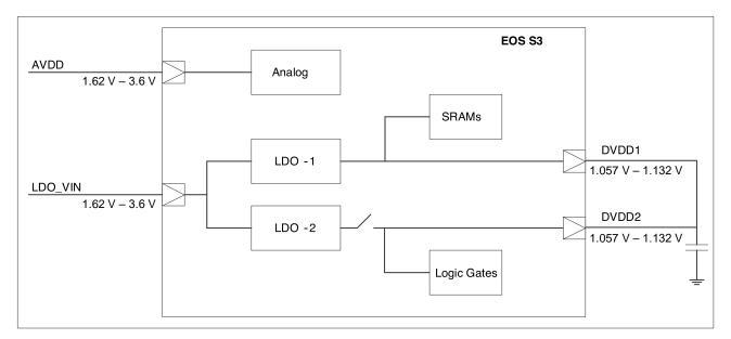
Figure 41: Use Case 2: Single Voltage Rail
