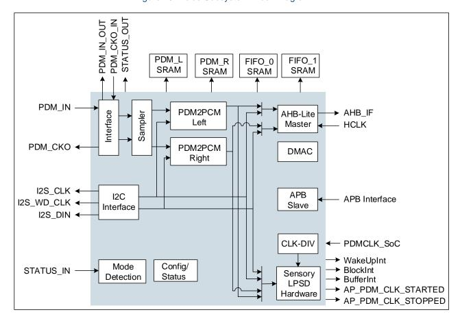
Figure 29: Voice Subsystem Block Diagram
