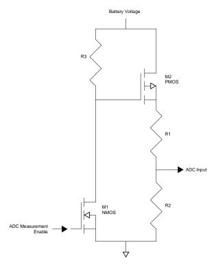
Figure 54: Example Voltage Divider Circuit
