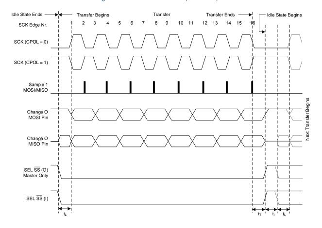
Figure 27: SPI Clock Format 1 (CPHA = 1)
