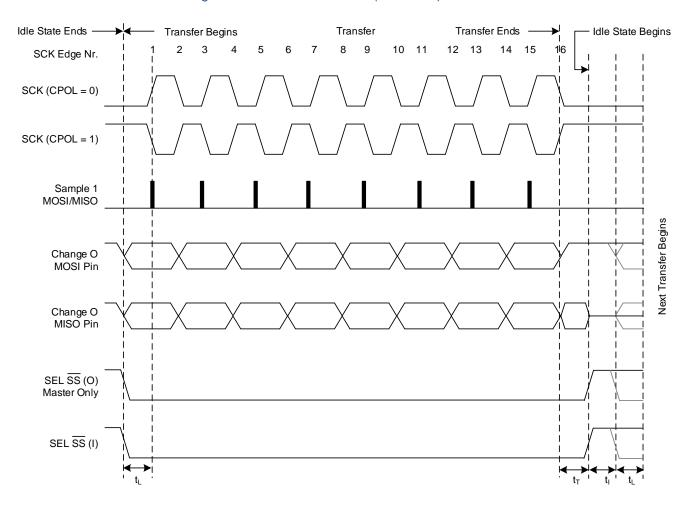
Figure 26: SPI Clock Format 0 (CPHA = 0)
