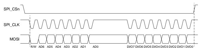
Figure 22: 3-Wire Basic SPI Read/Write Sequence (Mode 11)
