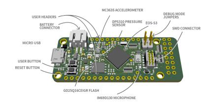
Unlike other development kits that are based on proprietary hardware and software tools, QuickFeather is based on open source hardware, is compatible with the Adafruit Feather form factor, and is built around 100% open source software (including the Symbiflow FPGA tools).
